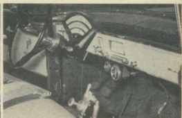
Floor mounted Moon fuel controls meter fuel from tank in trunk. Tach and pressure gauge have been added beneath dash.
